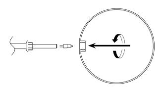
**3** Fix the ceiling plate (A) to the ceiling by using mounting plugs and screws suitable to your ceiling type. Guide the wires through the plate. Place or hold the lamp in an elevated position in such a way that the wires can freely reach the ceiling junction box.
